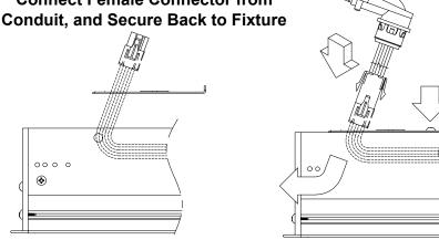
4: Push connectors into fixture as shown and secure 90° connector.
