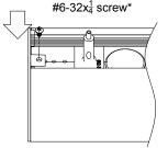
\* DO NOT over tighten screw. Hand Tightening is recommended.
