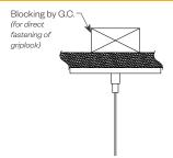
NON-Feed Suspension Point A/C Cable White Canopy 5" dia. Length: ASW5 - 5' length ASW10 - 10' length ASW20 - 20' length
