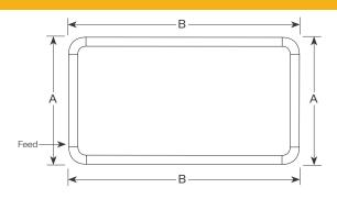
**PR** - Closed Rectangle, (4) straight lengths + (4)  $90^{\circ}$  corners Provide overall lengths: A' & B'; Diameter
