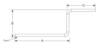
PZ - Open Z, (3) straights + (2) corners Provide overall lengths: A', B' & C'; Diameter & Angle of corners Example: 12'x6'x10'.D36XA90.PZ
