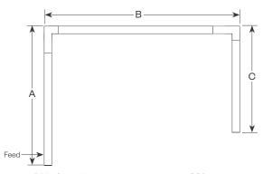
**PU** - Open U, (3) straight lengths + (2) 90° corners Provide overall lengths: A', B' & C' Nomenclature: A-B-C-PU
