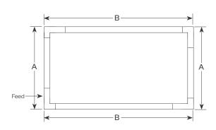
PR - Closed Rectangle, (4) straight lengths + (4) 90° corners Provide overall lengths: A' & B' Nomenclature: A-B-PR
