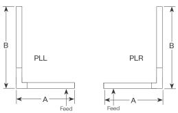
PLL - L Left, (2) straights + (1) 90° corner, leg right PLR - L Right, (2) straights + (1) 90° corner, leg left Provide overall lengths: A' & B'
