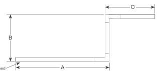
PZ - Open Z, (3) straight lengths + (2) 90° corners Provide overall lengths: A', B' & C' Nomenclature: A-B-C-PZ
