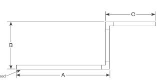
PZ - Open Z, (3) straight lengths + (2) 90° corners Provide overall lengths: A', B' & C' Nomenclature: A-B-C-PZ
