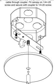
B: Install crossbar assembly into junction box. Thread
