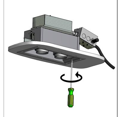
5. USE SCREWDRIVER TO TIGHTEN SCREWS. CLAMP WILL ROTATE IN TO PROPER POSITION TO KEEP FIXTURE IN PLACE WHEN TIGHTENING SCREWS.
