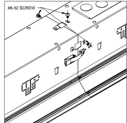
**C:** Once latched, secure fixture with #8-32 screws.
