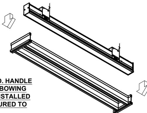
LIFT FIXTURE INTO SECURED GRID. HANDLE FIXTURE CAREFULLY TO AVOID BOWING AND/ OR FIXTURE DISTORTION. INSTALLED FIXTURE TO BE LEVEL AND SECURED TO GRID.
