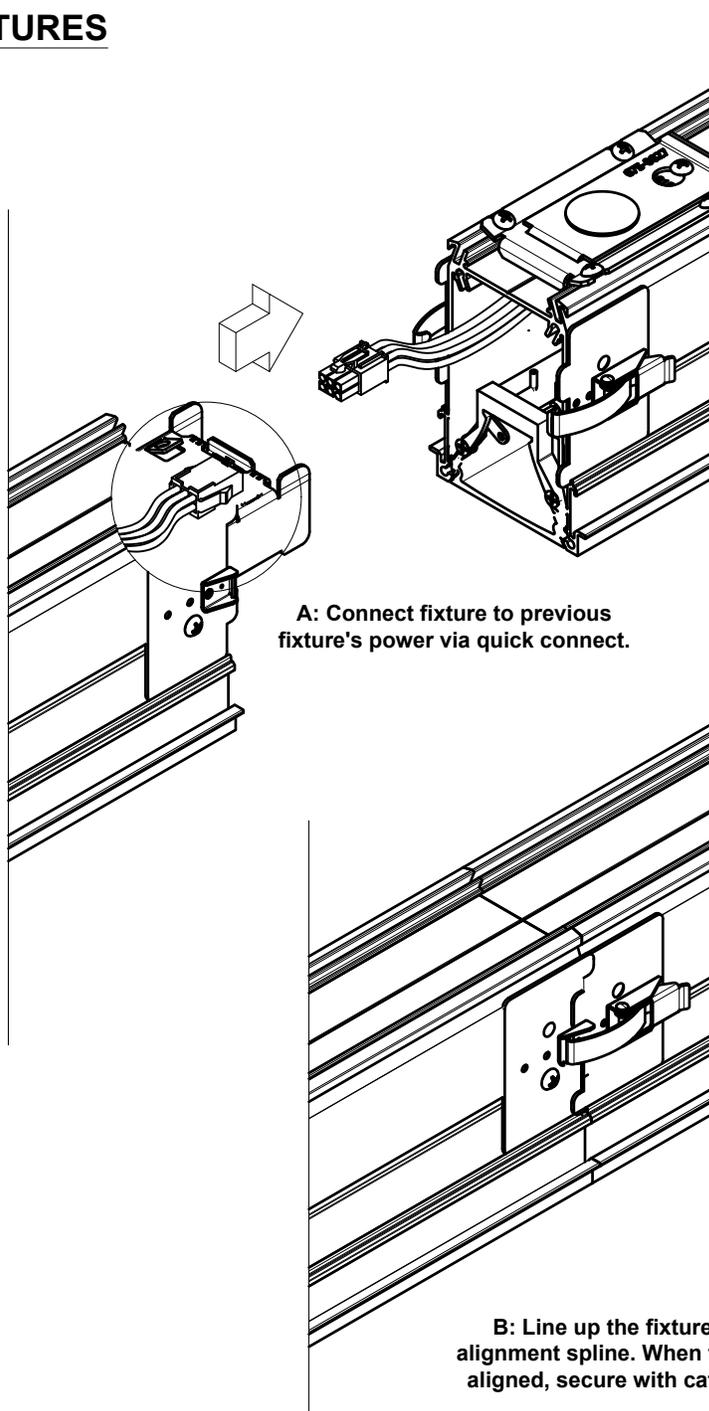
**A: Connect fixture to previous fixture's power via quick connect.**
