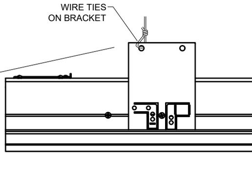
**C. TIE DOWN FIXTURE TO DECK WITH HOLES PROVIDED ON TOP SIDED OF FIXTURE OR ON TOP BRACKET.**
