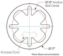
Note: Base accomodates existing bolt circles of 11.5" to 13" with up to 3/4" dia. bolts.
