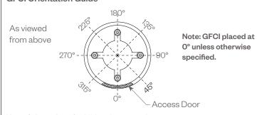
Note: Orientation of additional accessories must be specified when ordering.
