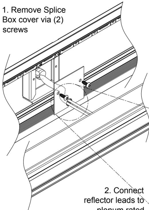
2. Connect reflector leads to plenum rated cable behind Splice Box cover
