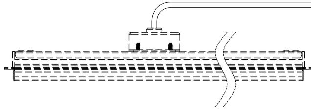
**4.** (Optional) Run plenum rated cable from multiple other fixtures into junction box and splice into feed from driver box
