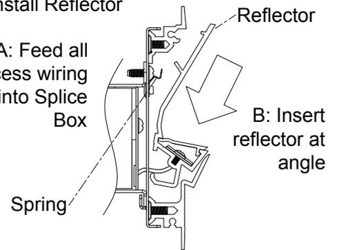
C: Press reflector Down and In until it "snaps" into spring
