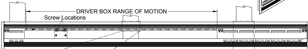
**5. Mount Fixture:** Secure fixture to structure (studs) via provided slots using **flat head screws** (by others). If fixture does not intersect any structure, blocking must be added (by others).
